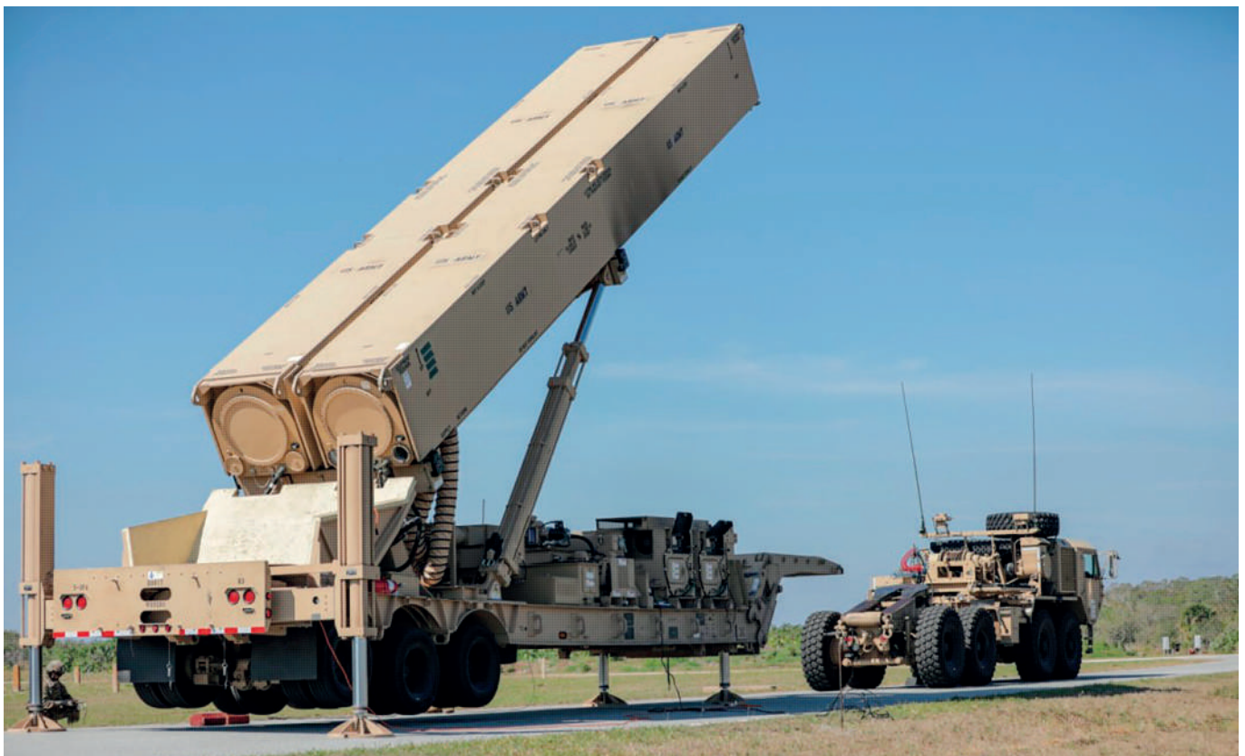
The US Army has finalized the development of the Dark Eagle system. This weapon combines a mobile ballistic launcher with the LRHW, a hypersonic glider and may have a range of around 2280 km. Pictured is the hydraulic launching system of the LRHW during Operation Thunderbolt Strike at Cape Canaveral Space Force Station, Florida, March 3, 2023 (photo: Wikimedia Commons / United States Government Works)
